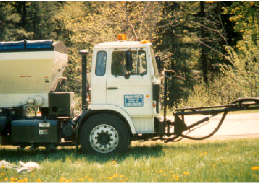
Figure 8. Spray-injection device—self-contained unit.
